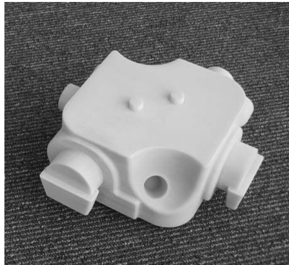
CAPForm SLS glass filed nylon Pattern
